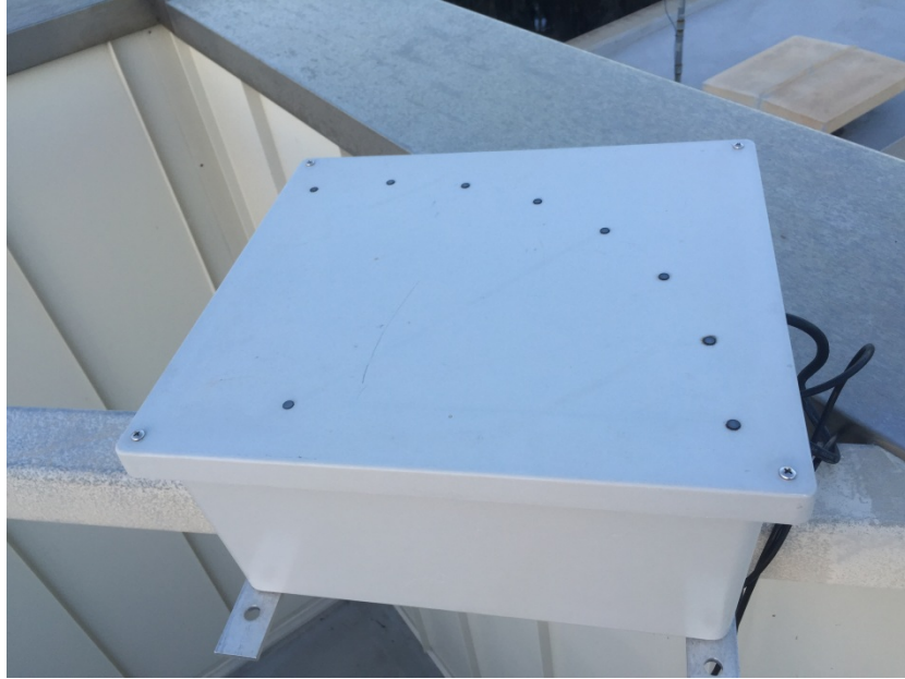
Figure 2 Cloud shadow Speed Sensor (CSS) contained inside a weather proof enclosure with dimensions 0.45 x 0.40 m. On the top of the enclosure is an array of nine phototransistors.
